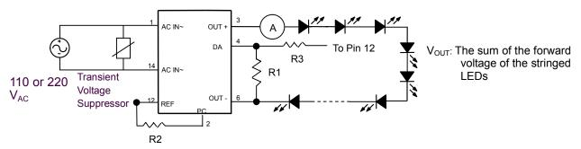
Note: There is no pin being connected to earth ground.
