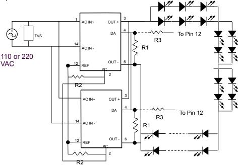
The selection of R1, and R2 is as defined as in the case of single string. Equivalently, the two MBI6001s are connected like piggy-back.
